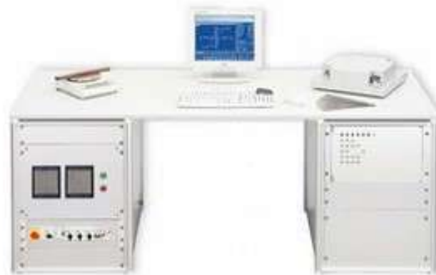
MPG 100 D Measuring Unit Epstein Frame 700 Windings
